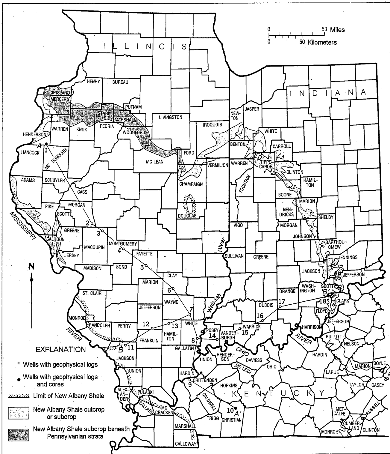
Figure 1. Map of Illinois, Indiana, and western Kentucky showing outline of the Illinois Basin based on outcrop, subcrop, and limit of the New Albany Shale (modified from Cluff and others, 1981). Map also identifies counties referred to in text and wells used in cross sections A-A' and B-B' shown in figure 3.
